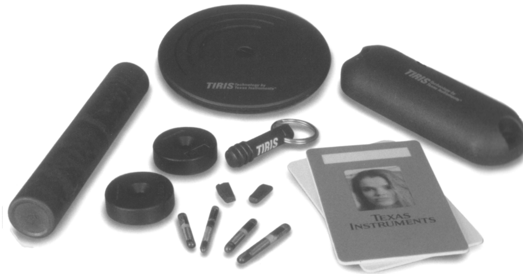
Figure 1. RFID tags – solid tags for containers/pallets; glass encapsulated tag for injection beneath skin; tag for moulding; tag integrated into key fob; tag integrated into I.D card (Source: Texas Instruments).
