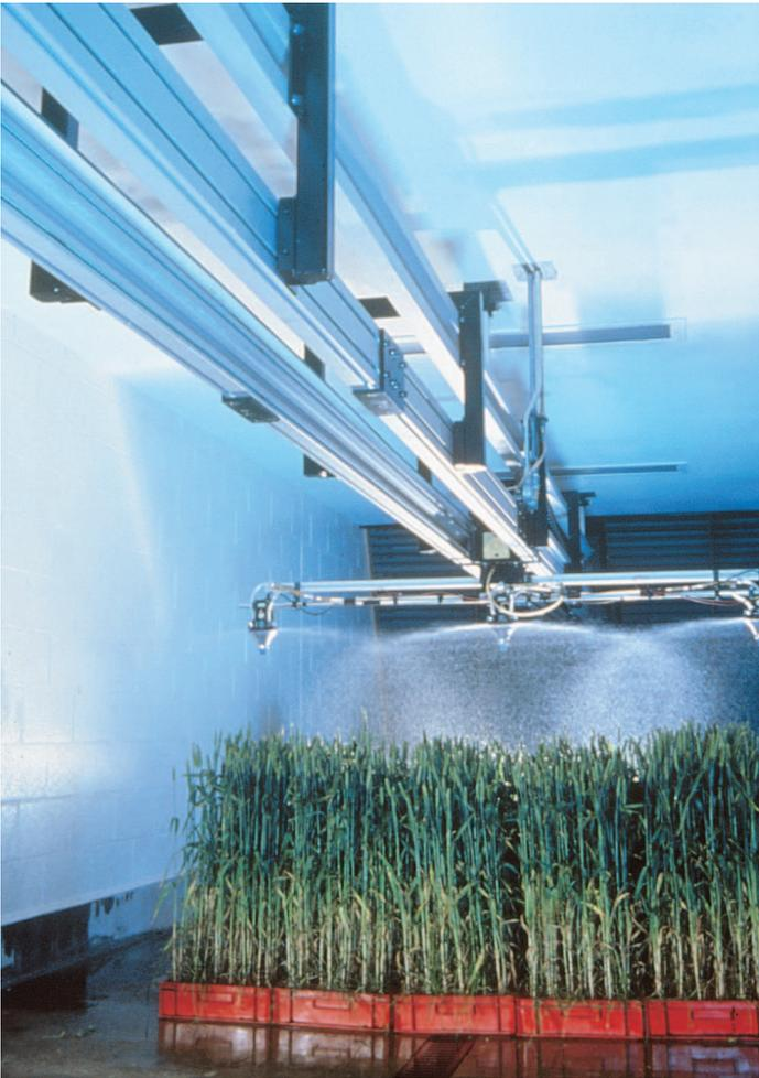
**The track sprayer at Long Ashton, which is used for the experimental application of pesticides under controlled conditions.**
