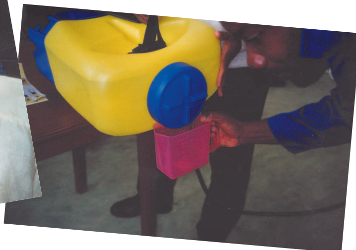
Measuring the leakage from a sprayer lid when the sprayer is "knocked over" onto the horizontal position (about 38 ml in 5 minutes).
