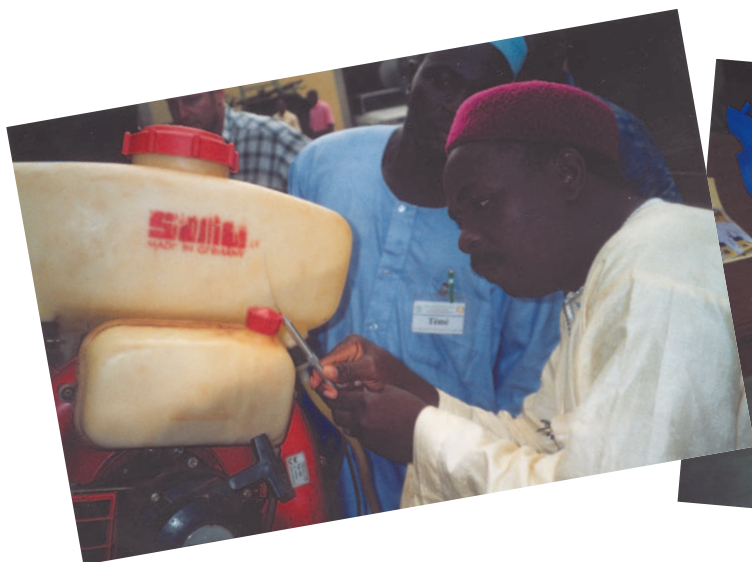
Examining engine speed of a motorised Solo mistblower using a "Vibratole" tachometer.
