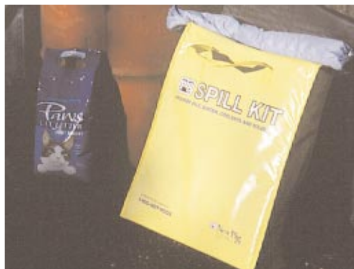
Figure 2. Cat litter and other inert material which can be used to absorb spills and drips.
